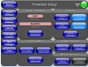
FIG. 47 Protected Setup page showing default values (MVP-8400)
